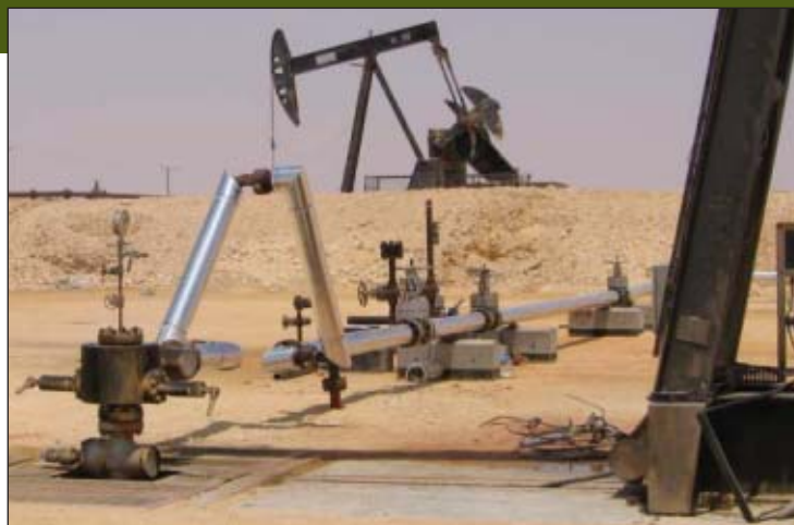
Steam injection in the Amal West pilot started during September 2007 (Fig. 2). Photo by Guntis Moritis.
